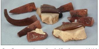
Spent Orton pyrometric cones from the kilns; the tan material (right foreground) is the cone pack base. Small cone numbers 01 (2152°F), 02 (2098°F), 03 (2068°F), and 04 (2008°F) were found.
