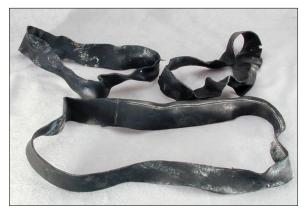
Intact rubber bands used for holding mold halves during slip casting. Cut from tractor tire inner tubes.
