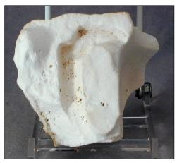
Mold fragment from a groove-handled creamer. Matching indents and knobs on the two faces of the mold halves were used for maintaining consistent alignment.
